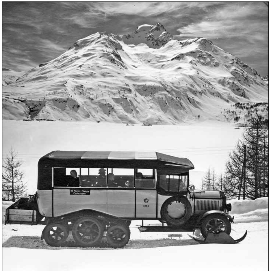
The larger, winterised St. Moritz - Maloja - Castasegna (Bergell) Postbus course as a caterpillar-driven snowmobile. Lake Sils and Piz de la Margna in the background. (Picture Sammlung Marco Jehli, Celerina)
